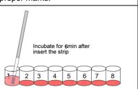
5. Insert the test dipstick into the wells with the "**Sample Pad**" fully dipped in to the mixture. Incubate for 6min at room temperature again.
